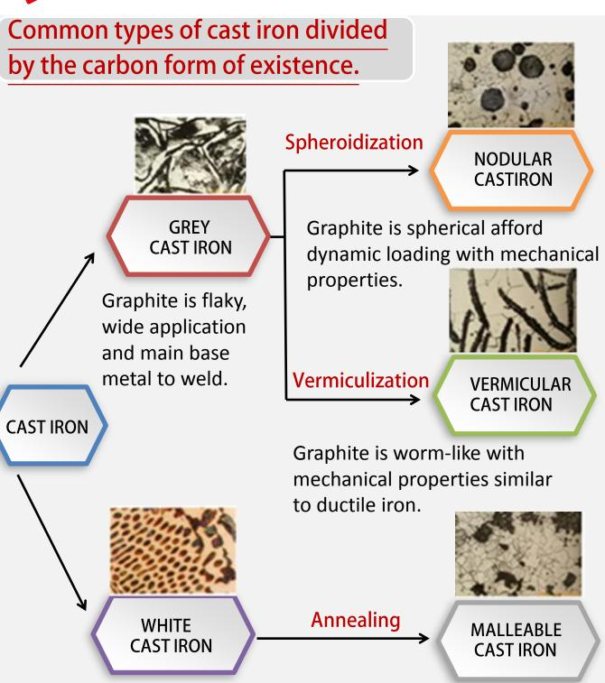
Carbon exist in the form of carburization. Hard and poor weldability.
